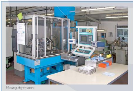
Honing is the last step before assembly. The finished, bearing rings run through a final process on machines co-developed by GRW for surface finishing of the raceways.
