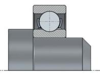
Right, Shaft radius smaller than r<sub>s min</sub>
