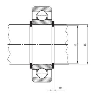
Assembly of a ball bearing with shaft circlips
