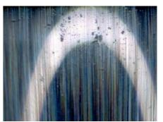
Indentations in raceway caused by particles
