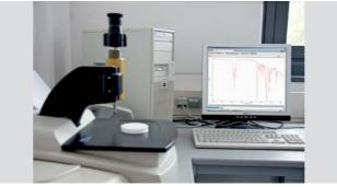
FTIR spectroscopy with ATR technology for non-destructive analysis of the quality composition of organic materials.
